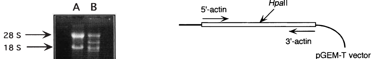
Fig. 4. Cloning of the internal standard plasmid for the competitive PCR analysis of cytoplasmic \beta -actin mRNA. For the construction of an internal standard applicable in primer competition, a new vector was constructed that contains the same primer-binding sites as the native cytoplasmic \beta -actin cDNA, but generates a 100-bp smaller fragment than the original PCR product. Since the size of this \beta -actin control plasmid is 3,305 bp (300-bp insert + 3,005-bp vector), 1 \mu\text{g} of this plasmid represents about 2.8 \times 10^{11} copies of this molecule.
